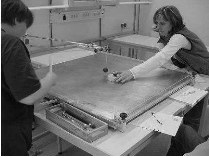
Fig. 1: Charged balls on an air flow table and parallel conductors for studying electric and magnetic forces.
