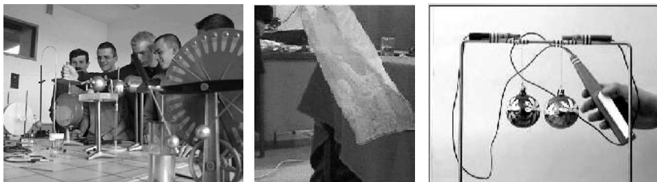
Fig.1: "Voltage" sources: a) Wimshurst's tribological machine (the right part of the photo), b) silk scarf taken from a wool coat doesn't hang vertically, c) piezoelectric gas-lighter used for "Christmas experiment".
