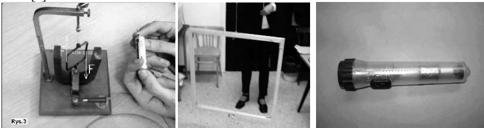
Fig. 3: AC electromagnetic current source, based on Faraday law, working also as electrical motors: a) a turning coil placed in the field of a permanent magnet [5], b) Helmholtz's coil - about 100 windings of 0.8 mm diameter wire wound on a wooden frame and turned around in the Earth magnetic field will create a few mV voltage; the same coil, supplied with DC current from car battery, turns slowly in the Earth field, c) hand-shaken lamp – the current is generated moving a magnet inside the coil (a toy made in China).
