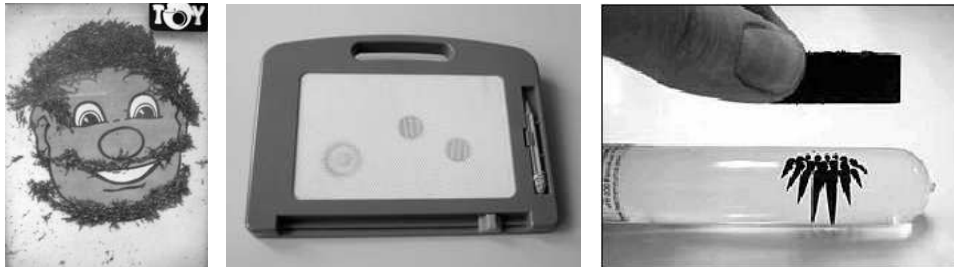
Fig. 6: Three devices to show the magnetic field lines. a) and old play with sub-millimetre iron fillings, b) a novel screen for drawing for children, made of micro fillings suspended in paraffin oil, the front screen is transparent; c) Ferro fluid cell [photo – www.teachersource.com ]
