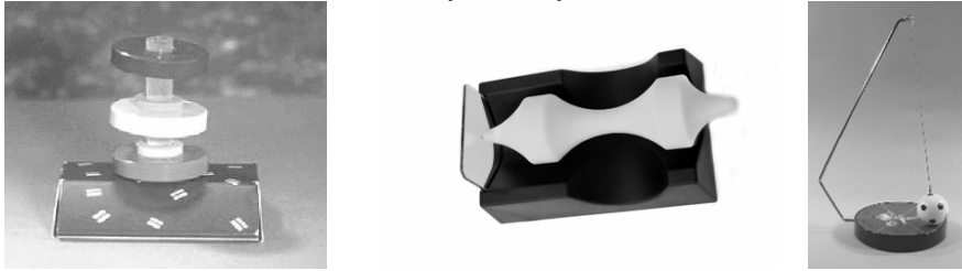
Fig. 4: Magnetostatic interactions: a) donuts, with poles on upper and lower bases are blocked in two directions by the stick; b) in the levitation pen, the poles of the same sign are placed in the base and on the external side of donut magnet in the pen; the repulsive interaction pushes the pen up (against the gravity) and left, against the barrier; c) in the roulette it is the cord from above which prevents the ball from flying apart.
