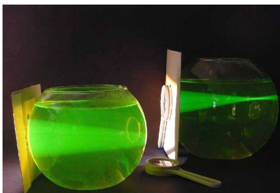
Picture 3: Water model of farsighted (left) and nearsighted (right) eye. Photo by G. Iskric.
